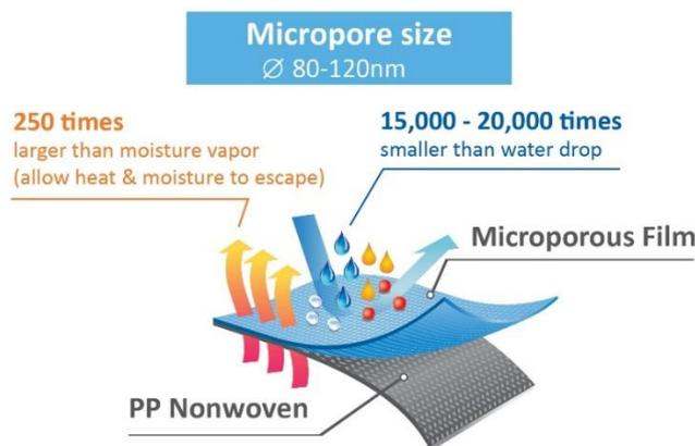
Figure 1. ULTITEC Fabric Construction
